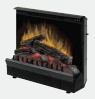
DFI2309 | 23" standard fireplace insert 23<sup>1</sup>/<sub>4</sub>" x 19<sup>1</sup>/<sub>2</sub>"x 10<sup>3</sup>/<sub>4</sub>" (WxHxD) 59 cm x 49.5 cm x 27.3 cm 120 Volts | 1,375 Watts | 4,695 BTU Available with expandable trim kit DFI23TRIMX
