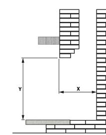
Note: Raise the G3.5 appliance by 2%" when using the 719BPB 4-Sided Backing Plate as the plate extends below the bottom of appliance.
